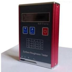
Roughness measurements can be useful to quickly identify locations where differences of wet slip resistance may exist. It can also be used to measure directional differences that might also create a slip hazard. In addition, the TR100 Surface Roughness Meter can identify changes in surfaces due to wear over time and soiling caused by traffic.
