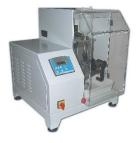
Instrument for determining depth abrasion resistance of unglazed ceramic tiles to ISO 10545-6
