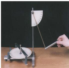
Impact tester is fitted with an arbitrary scale that is used to compare the results from different samples.
