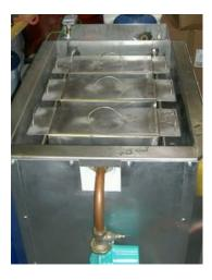
detergent solution Each container is fitted with a ware rack for easy handling of test samples Tank is heated with 3 kw (3 place) or 2 x 3kw (6 place) immersion heater and supplemented by a circulation pump Temperature is controlled to 77 deg C +/- 1 deg with a thermostat The unit is supplied with a digital thermometer and automatic constant water level system.
