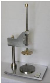
determines the test body deformation according to the Pfefferkorn Theory
